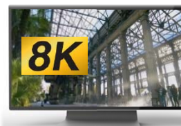
Figure 13. 27 inch 8K4K for signage (prototype) with 120Hz driving.
