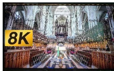
Figure 14. 80 inch 8K4K for monitor (prototype) with 120Hz driving.
